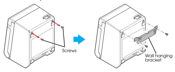
4. Align the holes in the wall hanging bracket with the screws on the wall, and hook it securely.
